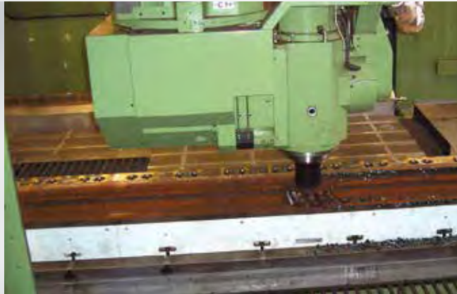
A ) Milling of the switch and stock rails to length 2 x 24 m
