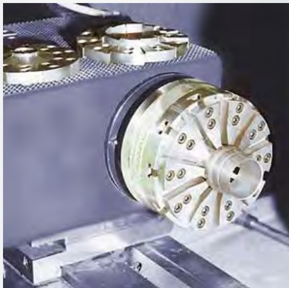
Circular grinding with permanent circular magnetic chuck. In this application upto 300 different workpieces can be machined using 4 sets of pole raisers.
