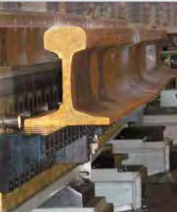
B ) Welding preparation of heart sections to length 2 x 5 m
