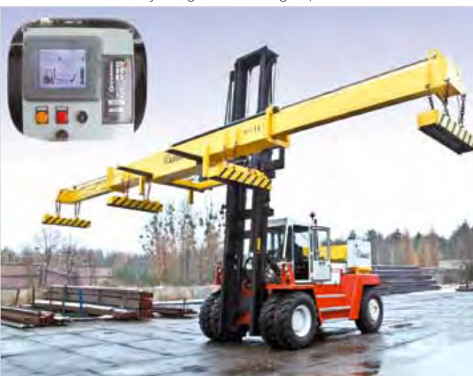
Telescopic beam with magnets on a fork lift truck. The power to the magnets is provided by a generator mounted on the truck
